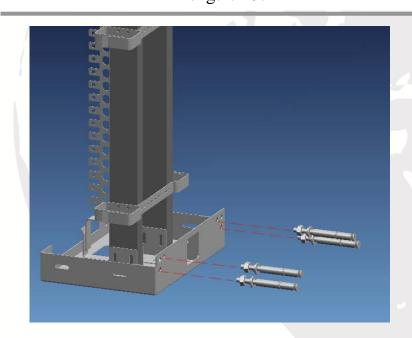
Distribution Frame is fixed with the Screws in the wall.
